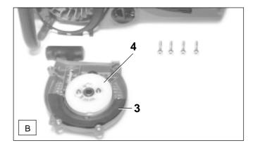
To get up to operating temperature faster (thus reducing wear and tear as well as fuel consumption), you can install a cover (B/3) inside the fan housing (B/4):
